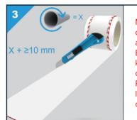
Measure the circumference of the service penetration and cut the Multitherm Bandage to size with a knife, as per the installation overview in the box. Remember to keep an extra length of at least 10 mm to create an overlap
