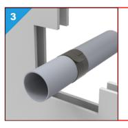
Wrap the required number of layers of Multiwrap around the service penetration.
