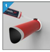
Seal the opening around the service penetration, according to the sealing method installation instructions. Openings up to 20 mm can easily be sealed with Multimastic SP firestop mastic, over a depth of 10 mm.
