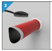
Make sure the service penetration is free from dust, dirt and grease.
